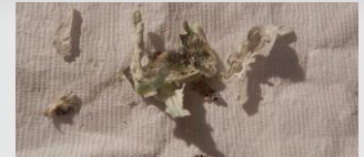
Hardened starch from outside of supply pump
